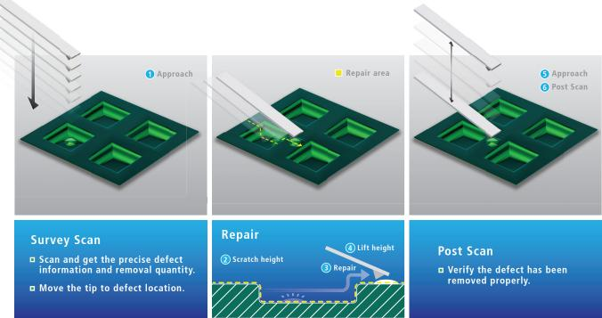
Following the repair, Park NX-Mask employsour non-contact AFM technology to conduct post-repair verification, generating nanoscale 3D topography and other critical metrology data such as surface roughness.
