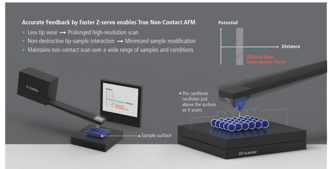
Unlike in contact mode, where the tip contacts the sample continuously during a scan, or in tapping mode, where the tip touches the sample periodically, a tip used in non-contact mode does not touch the sample. Because of this, use of non-con-
