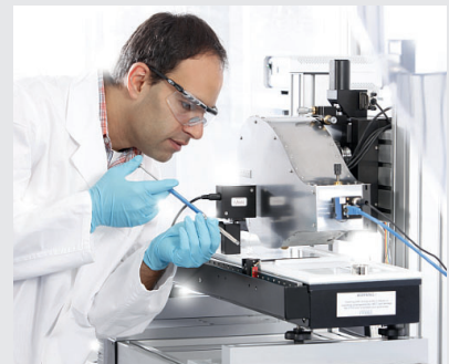
Monolayer experiment with NIMA trough
